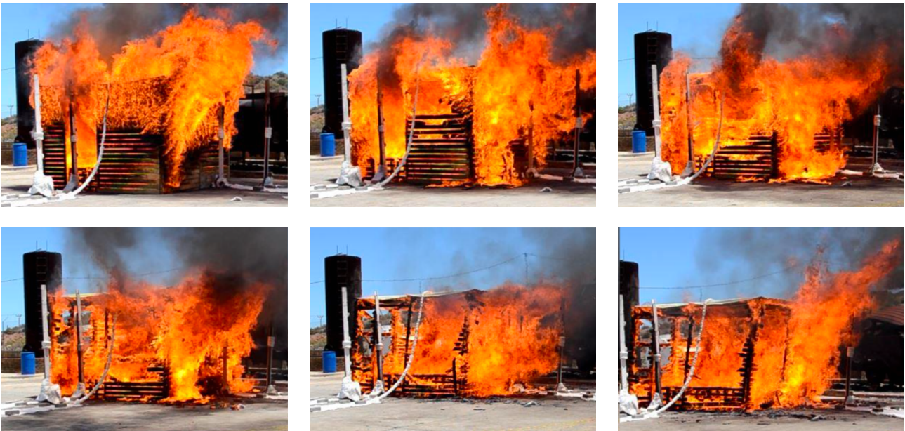
Figure 6: Timber plank wall and corrugated steel sheet roof shelter experiment conducted by the University of Stellenbosch
