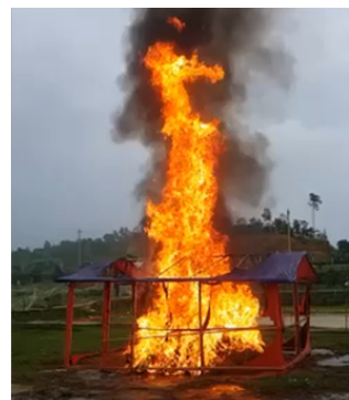
Figure 7: Photographs of fire experiments: (left) non-combustible enclosure experiment by University of Stellenbosch and (right) combustible enclosure tested by MOAS
