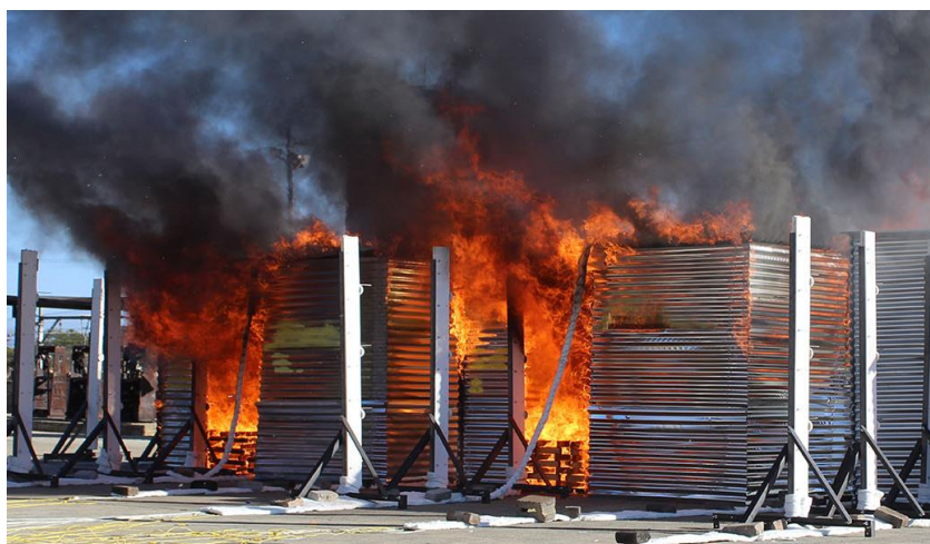
Figure 25: Non-combustible enclosure tested by Stellenbosch University [26]
