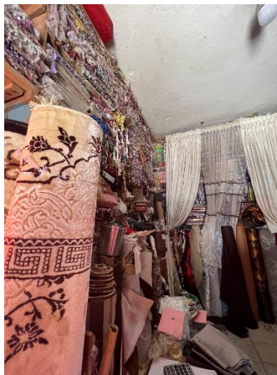
Figure 5: Combustible materials stacked high at a shop that survived the fire in a building on the perimeter of Waheen Market
