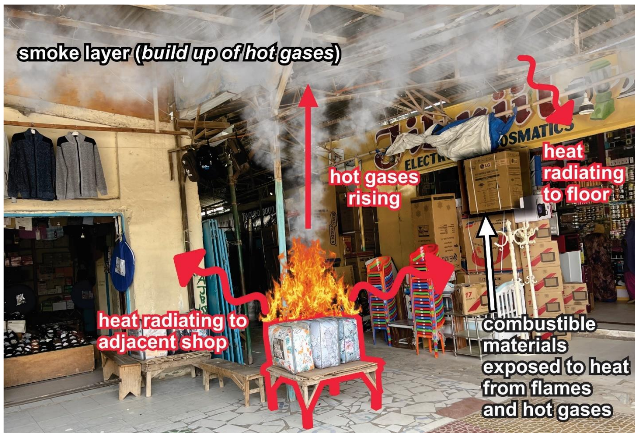
Figure 22: Mock-up of fire scenario in larger structure covering multiple shops
