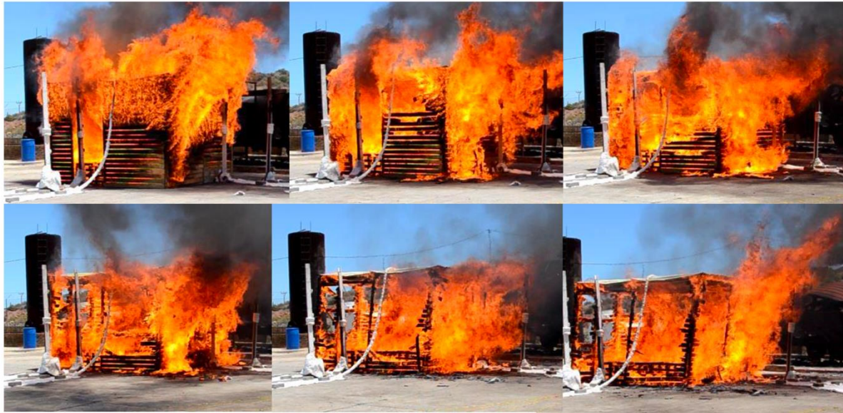
Figure 24: Timber plank wall and corrugated steel sheet roof shelter experiment conducted by the University of Stellenbosch [12]
