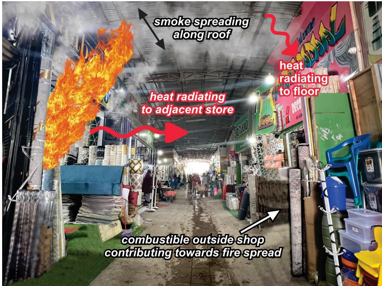
Figure 23: Mock Up of Fully Developed Enclosure Fire Scenario
