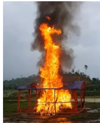
Figure 26: Combustible enclosure tested in Bangladesh [27]
