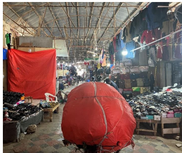
Figure 5: Combustible materials stacked high at a shop that survived the fire in a building on the perimeter of Waheen Market
